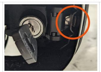
Lock the battery and remove the key.
