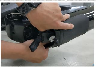
To make sure the battery is fully pushed into place, use both thumbs to push it in during the final stretch.
