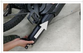
Carefully push the battery into the e-bike.
