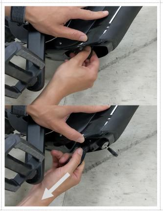
Unlock and carefully pull the Bosch battery out using the pull strap.
