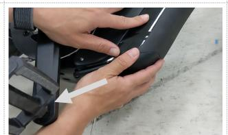
Unlock and remove the battery cover.
